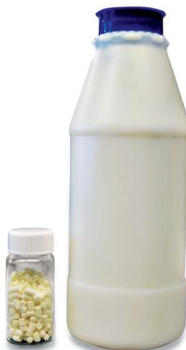
Yellow pellets composed of  $\text{CaWO}_4$  nanoparticles can be used to remove radioactive Sr from liquids, such as milk. Credit: Courtesy of Allen Apblett
